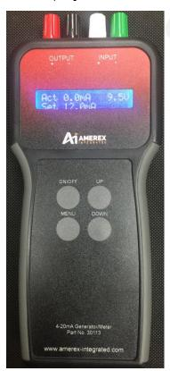
The 35113 has up and down membranes which allows the user to accurately adjust the output from the generator to a tenth of a mAmp.
