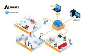
A recent addition to the AIMS family is the **Fire Panel Interface.** This is a panel that allows remote devices such as Sprinkler Flow switches, Tamper switches, Pressure switches and any other simple switch input to be connected to any fire alarm panel wirelessly. Thereby enabling a user to annunciate all the mechanical fire protection items on an existing or new fire alarm panel and having all the alarms managed in one place. The system being
