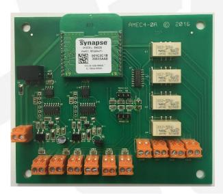
SNAP OS on-board Python interpreter provides rapid application development and over-the-air programming, while Atmel's low-power RF single-chip design saves board space and lowers power consumption. The modules provide up to 16 channels of operation in the ISM 2.4GHz frequency band.
