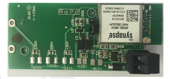
Once the node has been connected to the required open/closed contacts, power up the unit and connect to the mesh network by using the Portal commissioning tool.
