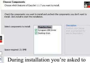
During installation you're asked to disconnect any Synapse USB devices. This is so the installer can load new drivers. Disconnect any Synapse USB devices and press Ok to complete the installation.
