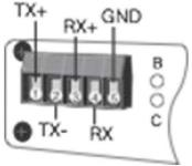
A terminal block is provided to which the transmit (TX), receive (RX), and ground (GND) wires can be attached. The factory default is set to 2-wire, but can be changed using the DIP switches
