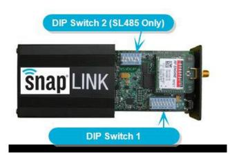
However, if you do not have access to a computer running EasySet, you can configure some communication parameters using the DIP switches located inside the unit.
