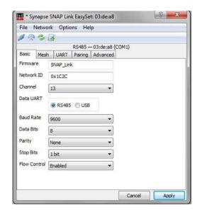
In this example we are attaching a device running at 9600 baud with 8 data bits, no parity, 1 stop bit, and with flow control enabled.
