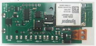
channels of operation in the ISM 2.4GHz frequency band. By default, the 30110 operating system automatically forms a mesh network with other nodes immediately on receiving power. No further configuration is necessary.
